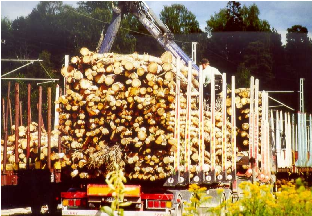
Figure 50 The reloading of logs from the lorry to the railway wagon (Foto: UPM-Kymmene 2000).
